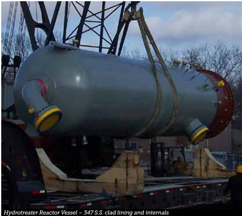
Hydrotreater Reactor Vessel – 347 S.S. clad lining and internals
